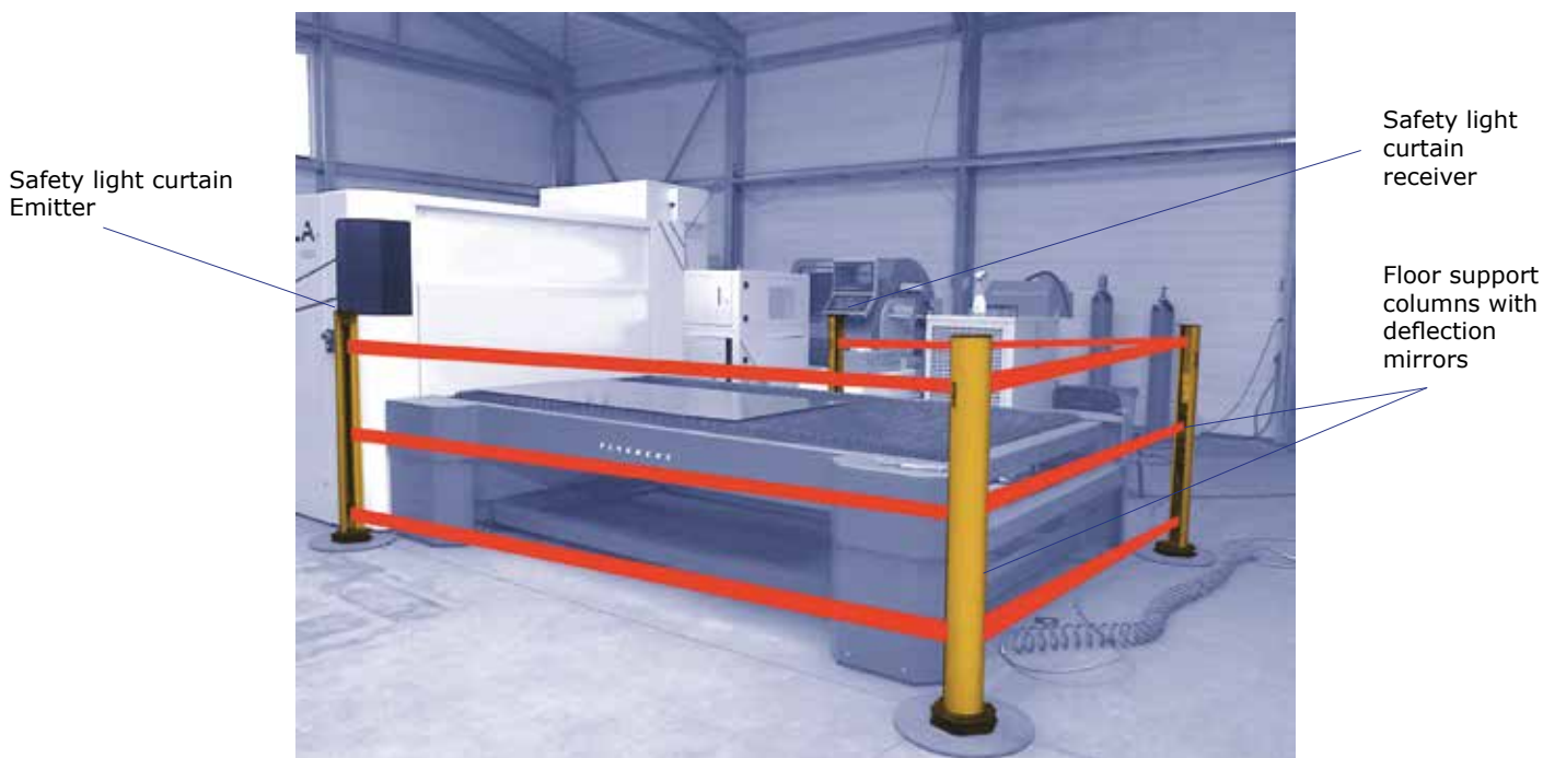
Fig. 26. Machine for laser cutting perimeter protection
