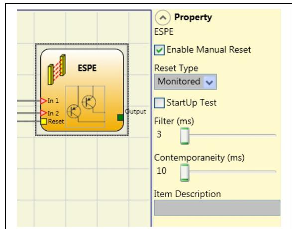
There are two types of reset: Manual and Monitored. When Manual is selected the system only verifies the signal's transition from 0 to 1. If Monitored is selected the double transition from 0 to 1 and then back to 0 is verified.
