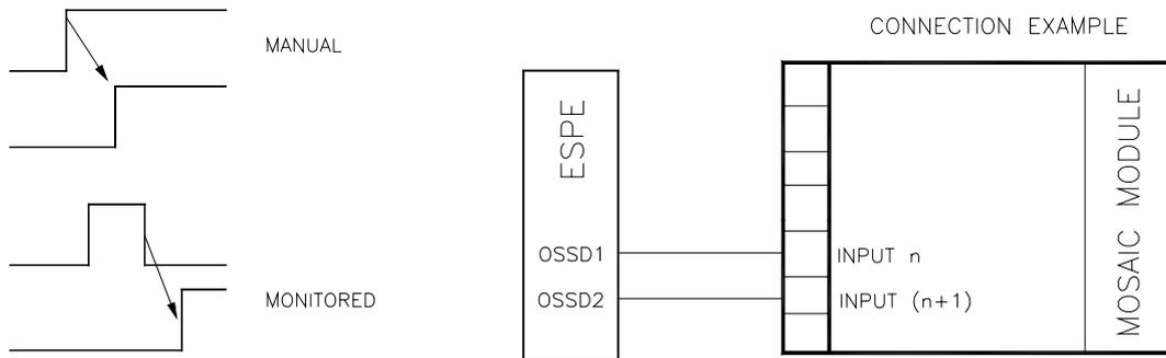
➔ **WARNING:** If the Enabled Reset is active, a consecutive Input have to be used. Example : Input 1 and Input 2 are used for the fuctional block, then Input 3 have to be used for the Reset Input.
