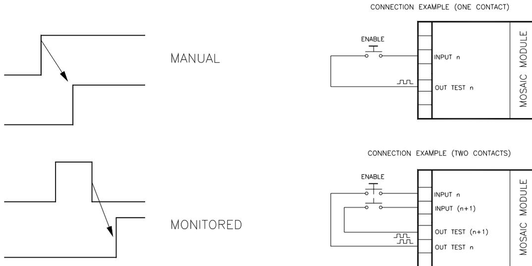
**Output test:** This is used to select which test output signals are to be sent to the component contacts. This additional test makes it possible to detect and manage any short-circuits between the lines. There is a choice of 4 possible test output signals, Test Output 1 ÷ Test Output 4.
