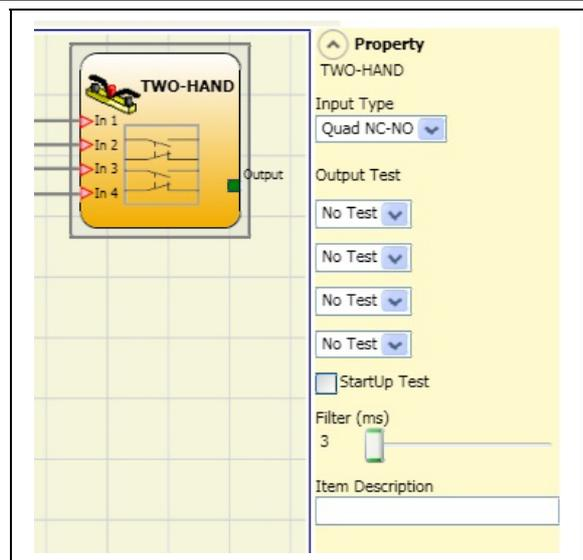
*Filter (ms):* This is used to filter the signals coming from the mode selector. The filter can be configured to between 3 and 250 ms and eliminates any bouncing on the contacts. The length of the filter affects the calculation of the unit's total response time
