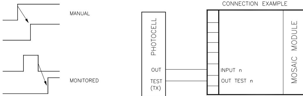
➔ **WARNING:** If the Enabled Reset is active, a consecutive Input have to be used. Example : Input 1 is used for the fuctional block, then Input 2 have to be used for the Reset Input.
