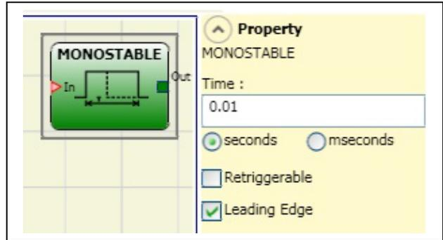
*Rising edge:* If selected, the output is set to 1 (TRUE) on the input signal's rising edge where it remains for the set time, which can be extended for as long as the input stays at 1 (TRUE).
