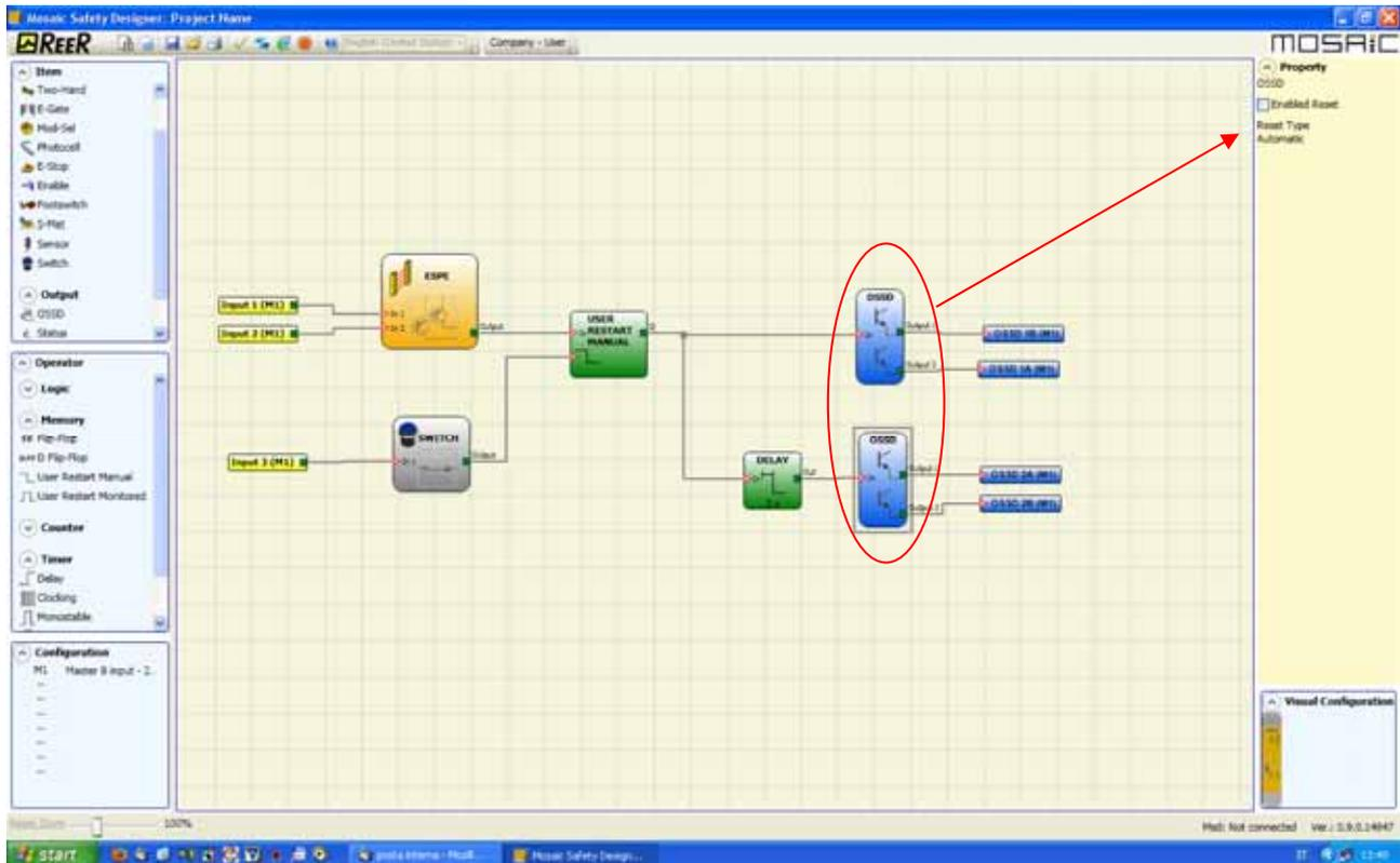
Figure 38 - Two outputs with one delayed (in MANUAL mode)
