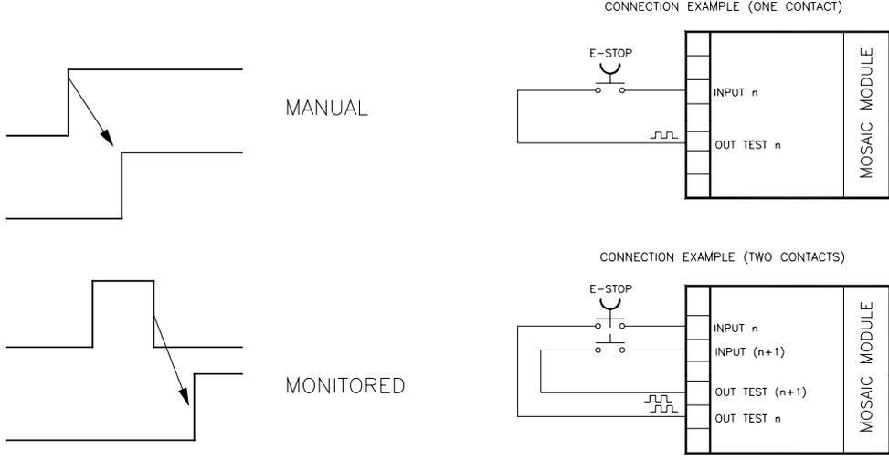
➔ **WARNING:** If the Enabled Reset is active, a consecutive Input have to be used. Example : Input 1 and Input 2 are used for the fuctional block, then Input 3 have to be used for the Reset Input.
