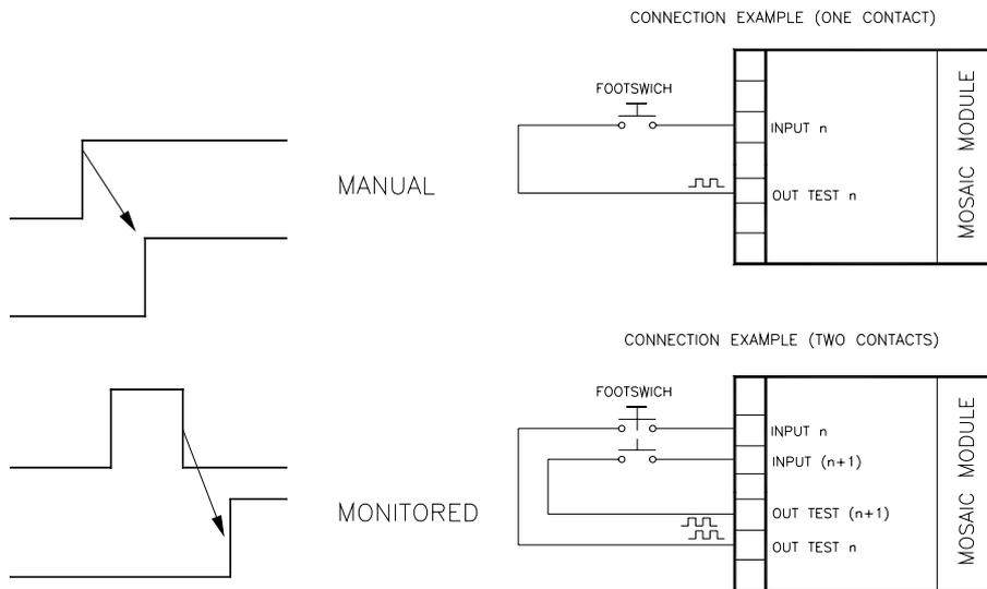
➔ **WARNING:** If the Enabled Reset is active, a consecutive Input have to be used. Example : Input 1 and Input 2 are used for the fuctional block, then Input 3 have to be used for the Reset Input.
