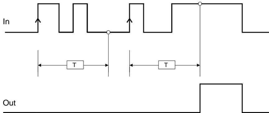
If not selected the logic is inverted, the output is set to 1 (TRUE) on the input signal's falling edge, the delay starts on the input signal's falling edge, at the end of the set time the output changes to 0 (FALSE) if the input is 0 (FALSE) otherwise it remains 1 TRUE.
