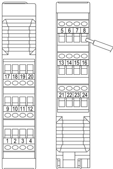
The MOSAIC system units are provided with terminal blocks for the electrical connections. Each unit can have 8, 16 or 24 terminals. Each unit also has a rear panel plug-in connector (for communication with the master and with the other expansion units).
