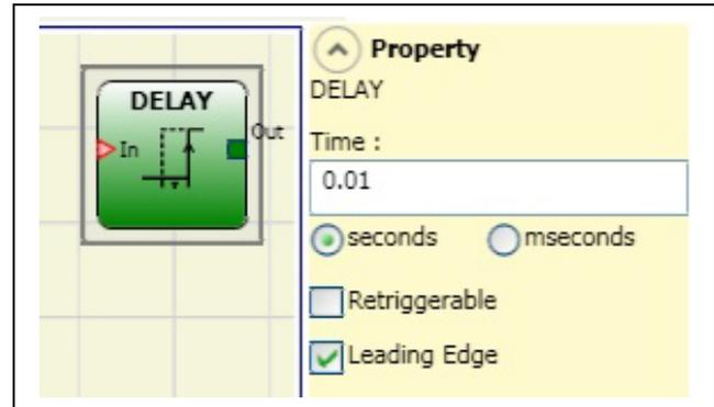
**Rising edge:** If selected, the delay starts on the input signal's rising edge at the end of which the output changes to 1 (TRUE) if the input is 1 (TRUE) where it remains for as long as the input stays at 1 (TRUE).
