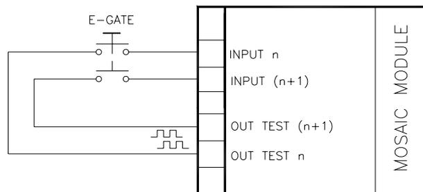
➔ **WARNING:** If the Enabled Reset is active, a consecutive Input have to be used. Example : Input 1 and Input 2 are used for the fuctional block, then Input 3 have to be used for the Reset Input.
