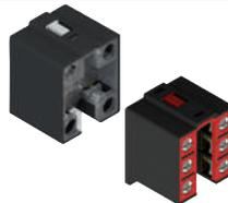
Contact blocks with captive screws, finger protection, twin bridge contacts and double interruption for higher contact reliability. Versions with gold-plated contacts available. Available in multiple variants with actuation by actuator or by solenoid.
