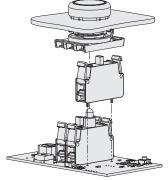
Versions with panel mounting of the EROUND series LED units with solder pin are available. If there is no wiring but a printed circuit, these LED units can be directly welded on the latter.
