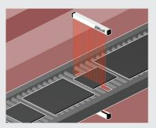
Measurement of the width and position of panels or sheets of material in transit on roller units or conveyor belts
