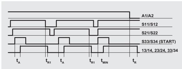
Legend: t\_MIN: Min. duration of start impulse; t\_c: simultaneity time; t\_A: response time; t\_R1: release time; t\_r: release time in absence of power supply
