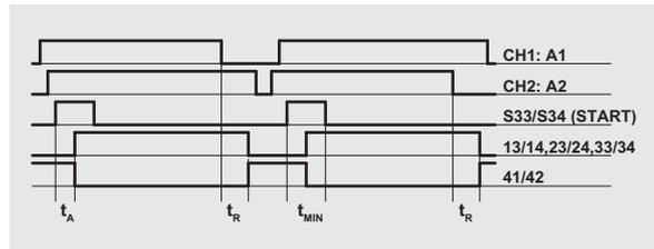
Legend: t\_MIN: Min. duration of start impulse, t\_A: simultaneity time, t\_R: response time, t\_R: release time in absence of power supply
