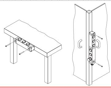
Thanks to the design with turnable modules, the control device units of the BN series offer the user many different options for fixing to the machine.
