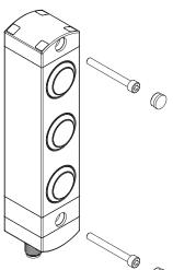
Each control device unit of the BN series is supplied complete with snap-on protection caps to be applied on the holes of the fixing screws. Not only do the caps prevent deposits of dirt from accumulating and simplify cleaning, they also prevent access to the fixing screws of the device, thereby offering increased protection against tampering.
