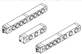
The control device unit is available in various configurations: for standard applications there are configurations with 3 or 4 devices, while configurations with 6, 7 or 8 devices are available for more complex applications that allow a larger number of control and signalling devices to be attached at the same location for the user.
