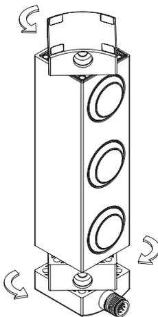
During installation, the fixing modules can be turned on the top and bottom of the device to enable variable orientation of the control devices.
