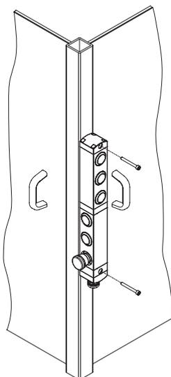
Thanks to the design with turnable modules, the control device units of the BN series offer the user many different options for fixing to the machine.
