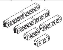
The control device unit is available in various configurations: for standard applications there are configurations with 1 to 4 devices, while configurations with 6, 7 or 8 devices are available for more complex applications that allow a larger number of control and signalling devices to be attached at the same location for the user.
