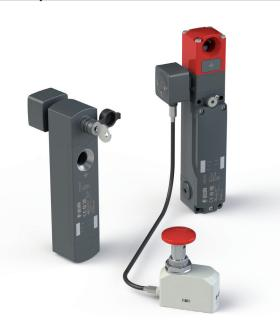
The remote escape release is operated via a flexible cable and facilitates remote unlocking of the safety switch in cases where conventional release devices (lock-type, by screwdriver, push button, etc.) are not easily accessible due to the configuration of the machinery.
