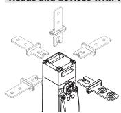
After loosening the 4 screws on the holding head, the holding head can be aligned relative to all four sides of the switch.
