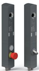
These switches are used mainly on machines where the hazardous conditions persist even after the machine has been switched off. Mechanical parts such as pulleys, saw blades, etc., could continue to move after the machine is switched off. Thus, the switches can also be used if individual guards are only to be opened under certain conditions.
