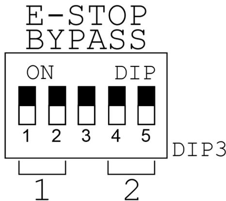
If the first two switches "1" and "2" are switched "ON" this bypasses the first emergency stop button connected. The two switches "4" and "5" bypass the second emergency stop button connected. The switches must only be operated when the BP gateway is OFF, in order to prevent incoherent input test signal readings.
