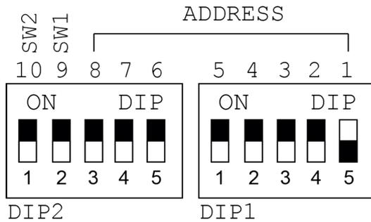
The two remaining switches (9 and 10) called SW1 and SW2 are reserved and not used for the safe address.
