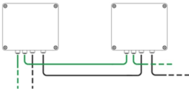
All P-Connect gateways are equipped with a double connector for the power supply of the device and for the fieldbus network connection. This makes it easy to install several P-Connect gateways in series by simply connecting the input and output connectors together. This feature was specially designed to reduce the time required for installation, disassembly and replacement of components during maintenance.
