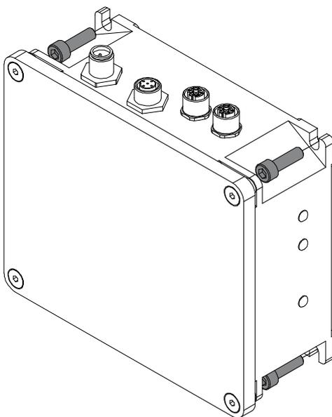
The device must always be fixed to the machine using at least two M6 screws with resistance class 4.6 or higher, with flat seating heads. The screws must have at least a number of threads engaged equal to or greater than their own diameter. The device must never be fixed with less than the specified number of screws.
